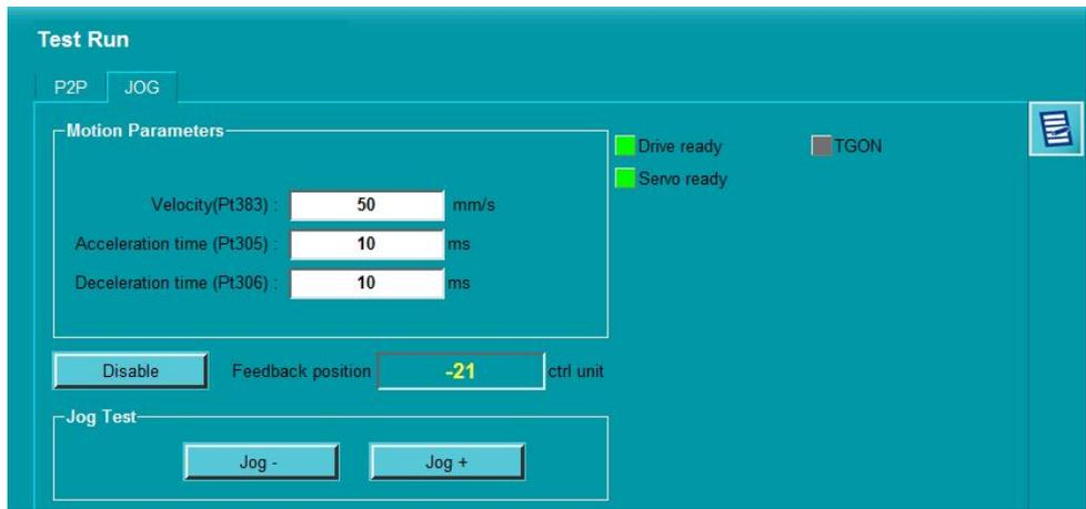
Figure 7.6 Low velocity jog on gantry mode
